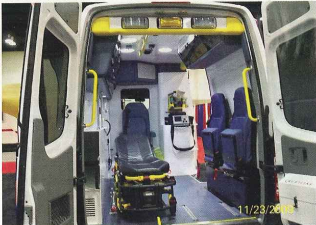
Interior with forward-facing seats stowed for loading or unloading. Note cardiac monitor and suction mounted in front of the front forward-facing seat.
