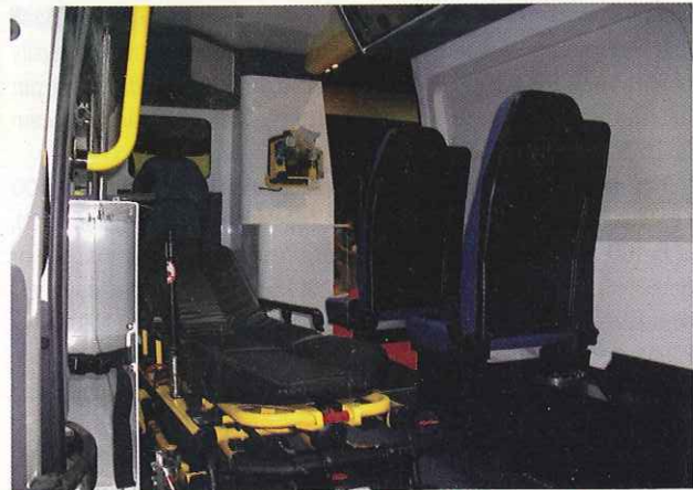
Seats prepared for transport: two forward-facing seats in position for transport plus one rear-facing seat (which contains a child seat within it).
